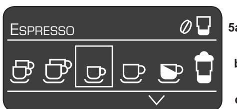
The status line **5a** in the display shows the name of the type of drink, along with the strength setting, e.g.  $\textcircled{0}$  and per-cup quantity, e.g.  $\text{\textcircled{1}}$ . The selection line **5b** shows symbols for drink selection. The arrows in the navigation line **5c** indicate the direction in which more menu levels can be found.
