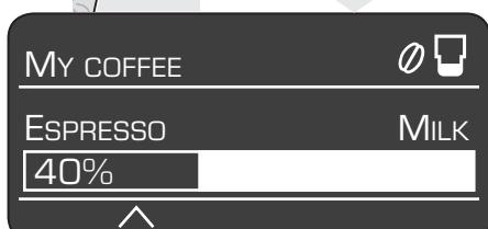
In addition to selecting the coffee strength and per-cup quantity you can choose the exact mix of espresso and milk for your own coffee setting **MY COFFEE** \*. The setting can be defined in 20% steps by turning the rotary knob 6.
